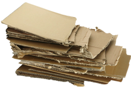
Corrugated Cardboard (Wavy center layer)
